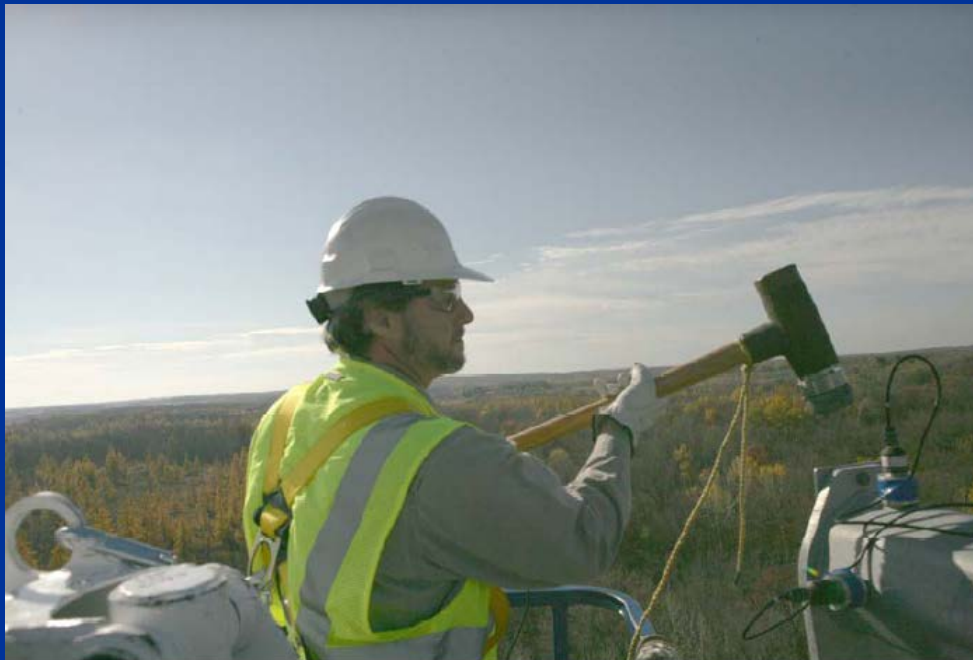
Figure 3 – Photograph showing a vertical impact of a davit arm with the modal impact hammer.
