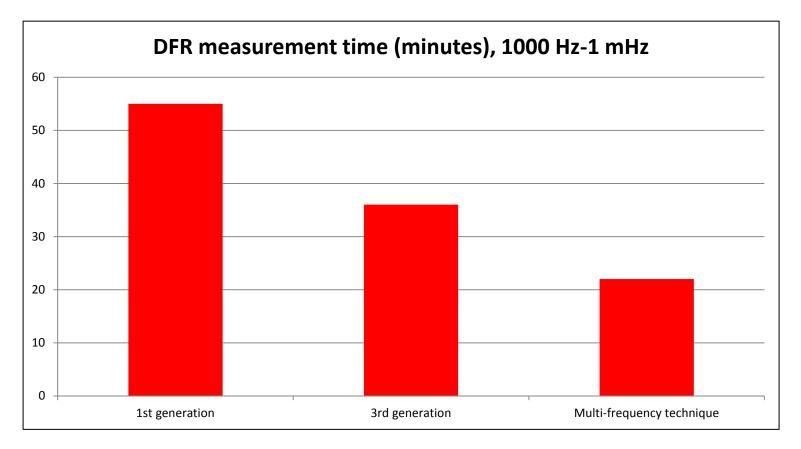
Measurement time with different frequency domain DFR technologies Frequency range 1 mHz – 1 kHz (20-30 C insulation temperature)
