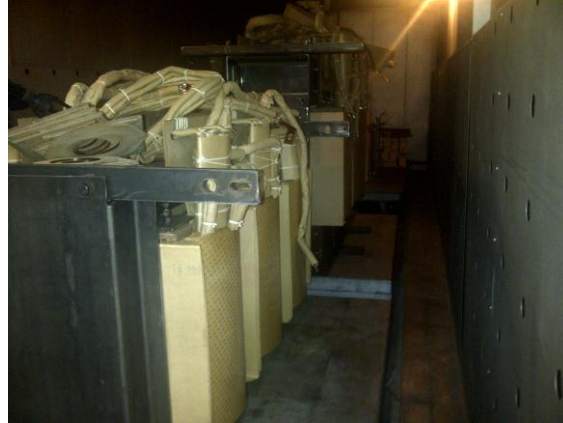
Figure 7 Core-winding modules set for thermal dry-out in the factory
